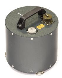
The CME-6111 seismometers combine the low-noise molecularelectronic sensing element (transducer) and the electrodynamic feedback, which results in very flat response over wide frequency range, high dynamic range and greatly improved time and temperature of the stability instrument The electrodynamic parameters. force feedback technique can be used for self-calibration or periodical selftesting.
