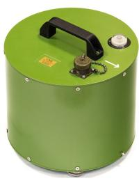
combine the low-noise molecularelectronic sensing element (transducer) and the electrodynamic feedback, which results in very flat response over wide frequency range, high dynamic range and greatly improved time and temperature of stability the instrument parameters. The electrodynamic force feedback technique can be used for self-calibration or periodical selftesting.
