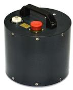
The CME-6011 seismometers combine the low-noise molecularelectronic sensing element (transducer) and the electrodynamic feedback, which results in very flat response over wide frequency range, high dynamic range and greatly improved temperature time and stability of the instrument parameters. The electrodynamic force feedback technique can be used for self-calibration or periodical selftesting.
